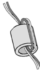
Figure 6. Loop Wiring Through Bead as Shown
